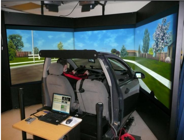
Figure 1. 180° field of view driving simulator.
